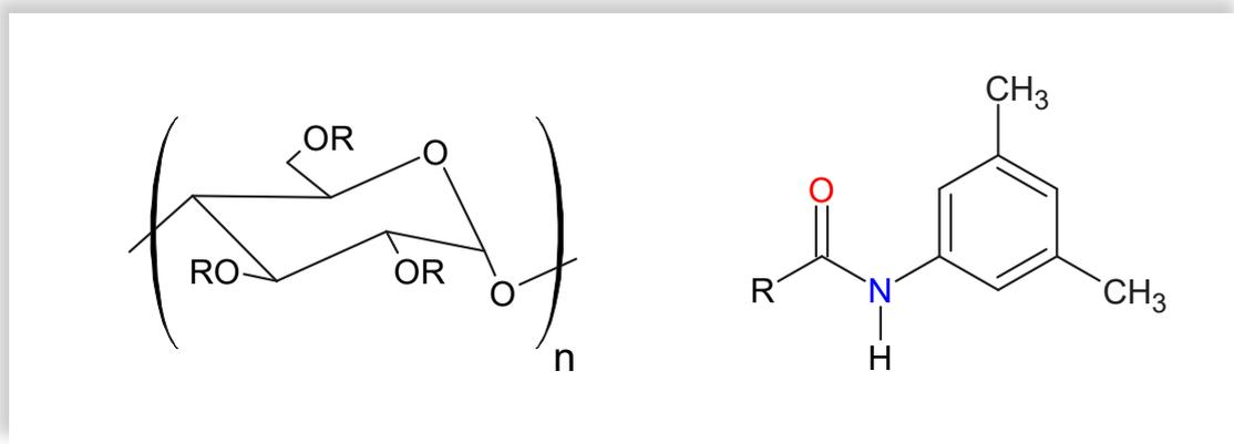
Retention on cellulose tris-(3,5-dimethylphenylcarbamate) could be explained by non-specific interactions such as  $\pi$ - $\pi$  interactions, hydrogen bonding and stereo-induced interactions.
