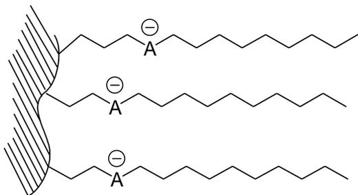
With an embedded acidic ion-pairing group, a Primesep 100 column requires no ion-pairing reagent in the mobile phase to retain and separate ionizable polar compounds. The ligand itself is a chain 12 carbons long (C12), and its acidic functional group has a pKa of ~1. Reversed-phase and cation-exchange functionality are assembled on one molecule to provide good reproducibility and stability.
